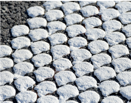
Multidot Featuring Multidot technology that maximises light return for exceptional wet night visibility. Certified for highways, it is ideal for high-traffic, nighttime areas. Available in white, it is applied by specialist extrusion machinery.
